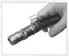
Move the clamp over the tube and the pillar of the coupling.
