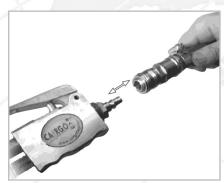
Put the connector of the air tool into the quick coupling. Press them firmly together.
