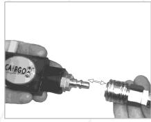
2. Put one of the valve connectors into the quick coupling of the air tool.
