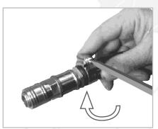
4. Turn the screw of the clamp to the right and fixate the clamp.
