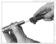
Slide the "Quick coupling hose pillar" into the tube.
