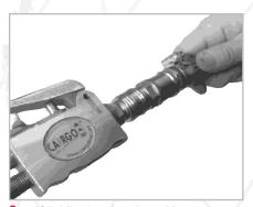
"Click", now the air tool is connected to the air tube.
